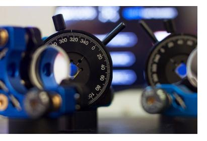
qutools' Entanglement Demonstrator is designed with educators in mind. It's the easiest and most reliable way to explain the complex phenomena of quantum mechanics by generating and analyzing polarization-entangled photon pairs.
