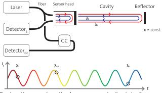
Tuning the wavelength also causes a similar interference pattern as moving the mirror. The absorption lines of a acetylene cell are used for precise wavelength control.
