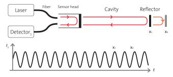
The interferometer is inspired by a Fabry-Perot-Interferometer. Fiber coupled laser light leads to a sensor head where 4% of the light is reflected back to the detector. The rest passes the cavity, is reflected and also guided to the detector. The graph shows the interference signal of a constantly moved mirror.
